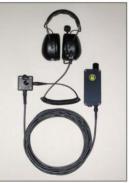
robust. The dive tenders unit can also be connected to an external speaker or voice recorder through an optional line-out connector.
