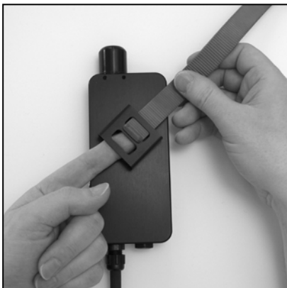
Figure 3: Attaching the transceiver unit to the head harness.
