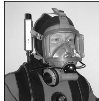
Figure 4, 5: Phone mounted on a full face mask.
