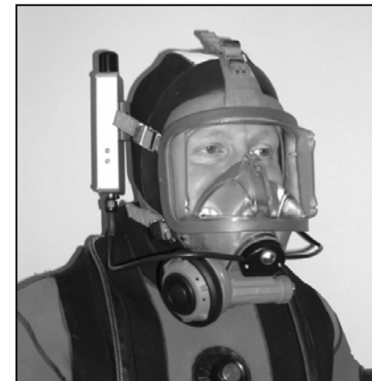
Figure 4, 5: Phone mounted on a full face mask.
